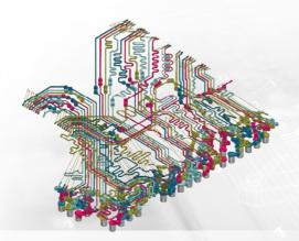
**SIwave – DC:** Engineers from Sarcina Technology LLC used ANSYS SIwave to extract DDR3 electrical models for both a PCB and its daughter card to analyze the performance of application-specific ICs used in Big Data applications and the Internet of Things.
