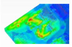
Current flow and thermal analysis simulations once performed separately can be combined in a multiphysics-based board-level electrothermal cosimulation via linkage between SIwave and ANSYS Icepak.
